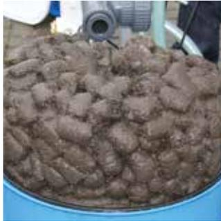
FIBALON® wwt has an excellent selectivity of 10 µm and is very easy to dispose. If outstanding filtration results and consistent filtration qualities are in the focus, FIBALON® wwt is the best choice. FIBALON® wwt guarantees also a pressureless filtration.
